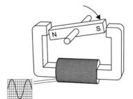
The natural waveform produced by a generator is AC, not DC
