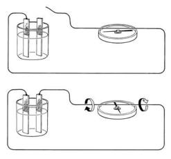
Oersted discovered that an electric current produces a magnetic field. But it was not *along* the wire as everyone expected but *around* it.
