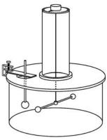
Coulomb measured the force of electricity with a fine piano wire.
