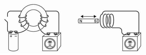
Faraday (and Henry) found that it was a *change* in a magnetic field that produced electricity. The needles twitched when the current was either turned on or off or when the magnet was moved.
