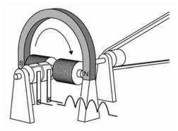
To avoid AC, early electrical generators used contacts to "rectify" the output. Although it didn't produce a steady current, at least it flowed in one direction only.
