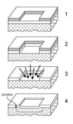
Hoerni's planar process, one of the most important inventions of the 20<sup>th</sup> century. In step 1 a photosensitive layer is exposed to light through a mask. In step 2 the oxide layer covering the silicon wafer is etched away in the exposed area. After the photosensitive layer is removed, impurities are diffused through the opening (step 3), thus forming a protected junction underneath the oxide. In step 4 the opening is closed by growing more oxide.
