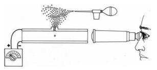
Millikan's oil-drop experiment, with which he determined the properties of a single electron.
