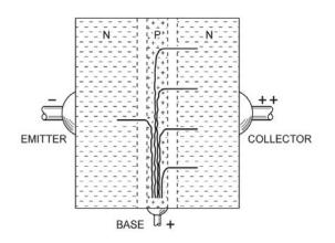
The Junction Transistor. There are three layers, with the center one (the base) doped oppositely from the outer ones. The baseemitter junction is a forwardbiased diode and a current flows. But, because the base is very thin, most of the carriers (electrons or holes) are swept away to the collector and never reach the emitter. Thus a small current controls a much larger one and the device has a "gain".
