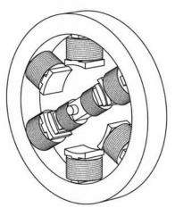
In his revolutionary AC system Tesla used multiple wires with the voltages staggered in time. The inner part, the rotor, was simply a piece of iron with a coil that became a strong electromagnet with rotation. No contacts were needed.
