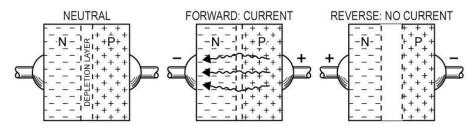
The Diode (or Rectifier). When P and N-doped regions are adjacent, some electrons fill holes, forming a no-man's land (the depletion region, left). With a voltage applied in the forward direction, the depletion region narrows until it is small enough that a current can flow (center). If the voltage is reversed, the depletion region widens and no (or very little) current flows (right). Thus a diode conducts in one direction only.
